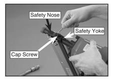
**Figure 6.** Loosening cap screw for depth adjustment.
